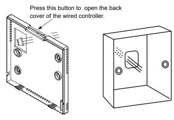
2. Fix back cover to the holder. After that, connect communication wire to CON1 port of wired controller. Finally put the front cover of wired controller to back cover to complete the installation
